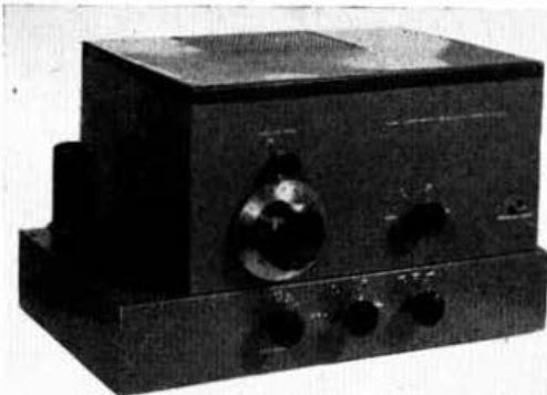
Front view of the T.V.I.-proof p.a., showing panel controls: Left to right (top) p.a. tank tuning and, immediately above, harmonic trap; tank-coil-turret band switch; (bottom) p.a. grid tuning; grid-coil band switch; and "Net-QRP-QRO" switch. The clamper valve can be seen on the left of the chassis.
